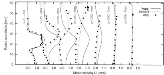
Figure 4: Mean axial velocity: comparison with experiment.
