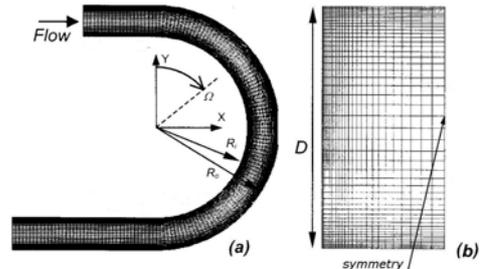
Figure 10: Numerical setup of U-duct channel.
