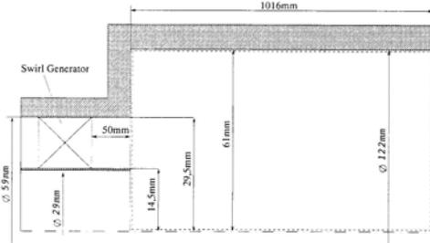
Figure 2: Description of combustor geometry ( $S = 0.45$ ).
