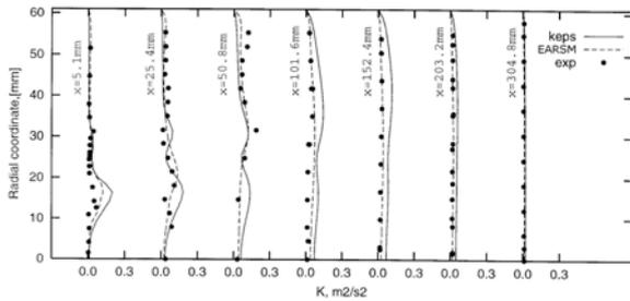
Figure 7: Turbulent kinetic energy: comparison with experiment.
