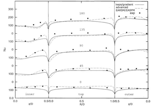
Figure 15: Local Nusselt number obtained using Low-Re  $k - \epsilon$  model and advanced EARSF.
