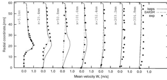
Figure 6: Mean tangential velocity: comparison with experiment.
