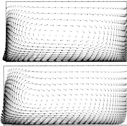
Figure 12: Secondary streamlines by  $k - \epsilon$  (above) and advanced EARSF (below).
