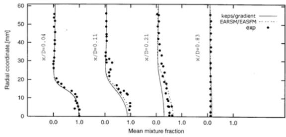
Figure 8: Mean mixture fraction: comparison with experiment.
