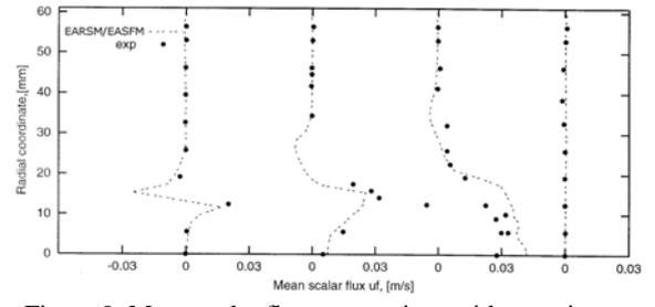
Figure 9: Mean scalar flux: comparison with experiment.
