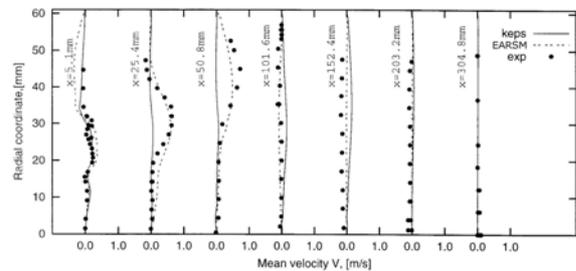
Figure 5: Mean radial velocity: comparison with experiment.
